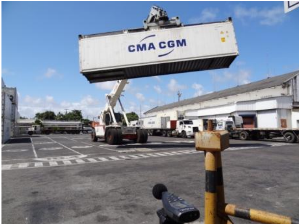
Figura 25 - Guindaste Reach Stacker
